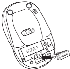
Fig. 6. Fitting the receiver into the mouse case
